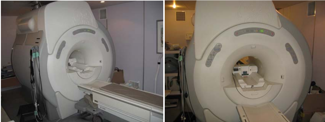
2006 Upgraded GE Signa CV/I 1.5T MRI with Excite 12
